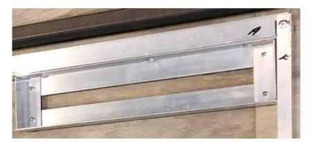
Rivet a tray to each side (A & B), and butted up against part G, with 3 rivets in the side and one on the end.
