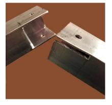
Cut the top of square stock piece B to allow it to slip into the notch of piece A.
