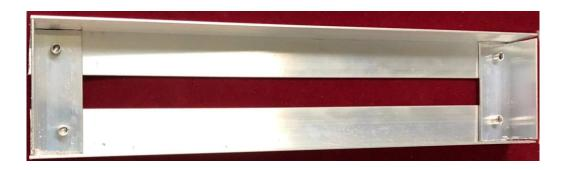
Use two pieces of 12" long and two 2¾" long to construct each of the 4 trays as shown above. You can also flatten a 2¾" long piece to add in the middle for better strength if desired but I elected to skip that.
