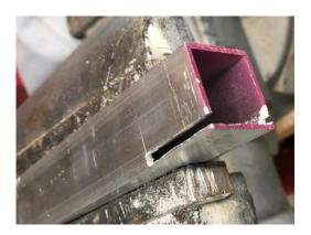
Bend the cut tab outward 90° (I bent this one in - but bent the rest out when I realized it was a better idea.)
