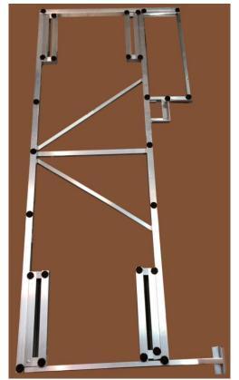
Place numerous stick-on durable furniture pads to the bottom. Be sure to place a pad over each rivet and each corner.
