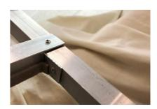
Cut 1" deep notches into the corner of one end of piece G. Bend the side out 90°. Rivet into place with rivets top and side.
